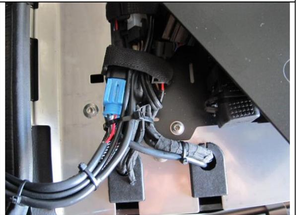
If a mobile radio is used, the receiver will need to be relocated to the LH saddlebag, not only for reasons of space, but also weight distribution. The FMS Accessories Radio Receiver Relocation kit includes a special mounting bracket along with radio power cable extension complete with BMW connectors, grommets and all needed hardware.
