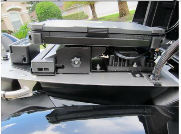
The lighter socket attached to the plug bracket is not easily transferred. Many agencies prefer to utilize that plug for powering a dual USB outlet available from FMS Accessories, complete with the mating BMW connector.
