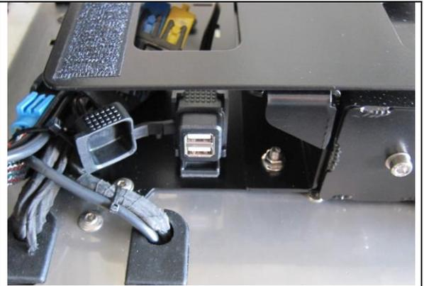
**Note:** Laptop chargers can be very consumptive ... most are LIND chargers with a maximum rating of 15A. It is recommended to utilize the FMS Accessory Laptop Charger Relay that will allow the LIND charger to **only** be powered when the ignition is ON, thereby preserving needed power in the auxiliary battery during violator stops when ignition is OFF.
