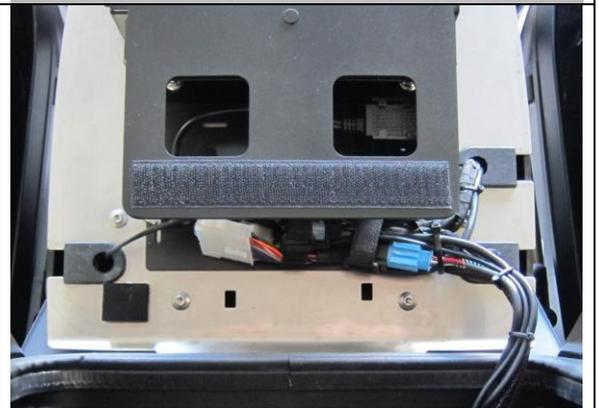
Ensure that cables flow freely up into radio box lid. Carefully observe the movement of the cables as you open and close the lid to ensure that cables do not "kink" or get pinched.
