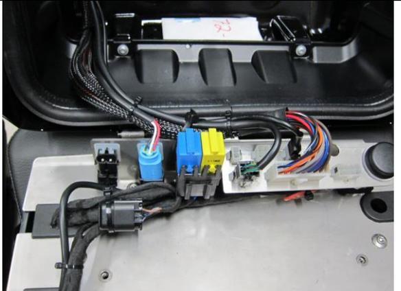
**Note:** it is helpful to place dots on the two-conductor plugs to aid identification (ACC I, II or III).
