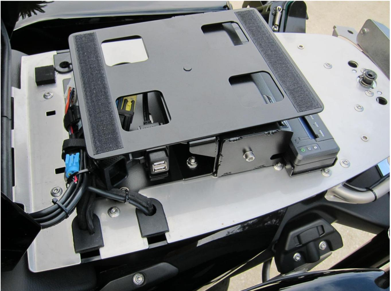
FMS Accessory laptop mounting is available with your choice of generic base plate or FHP base plate. The FHP base plate has mountings for a Rocket router as well as card scanner. The generic base has slots for attaching cables and other items such as laptop power supplies, etc. Both work well – the generic base was introduced to reduce weight and provide more convenient mounting locations / cable tie-down points.
