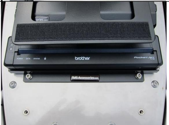
If the FHP bracket is used, the card scanner can be attached to the rear of the bracket / the Rocket router is attached at the front, using M5 self-clinching studs and serrated nuts. Note that the bracket was originally designed to attach the card scanner with the two mounting screws, but during testing, it was determined that those mounts were too fragile. It was better to attach the card scanner with locking Velcro.
